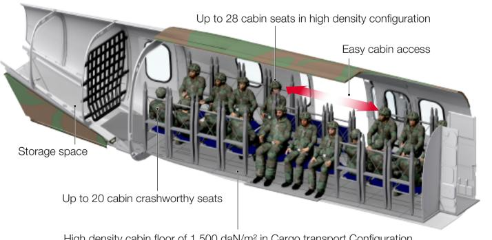
High density cabin floor of 1,500 daN/m<sup>2</sup> in Cargo transport Configuration
