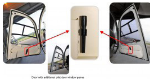
Door with additional pilot door window panes
