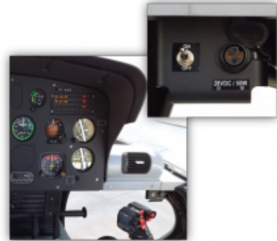
AS350 28 VDC outlet in the panel
