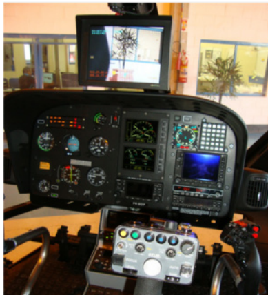
EC130B4 instrument panel with Flir System.
