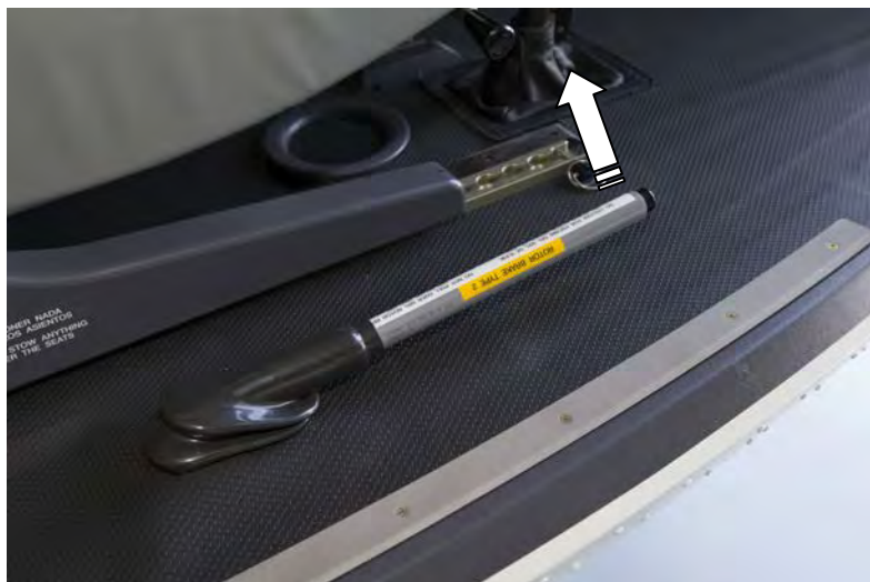
For activation press button on top of the lever and pull
