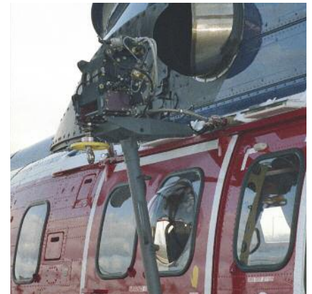
Class 1 hydraulic hoist 75 m / 272 kg
