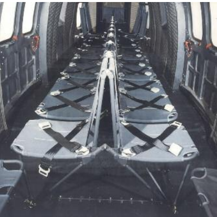
20 troop seats installation
