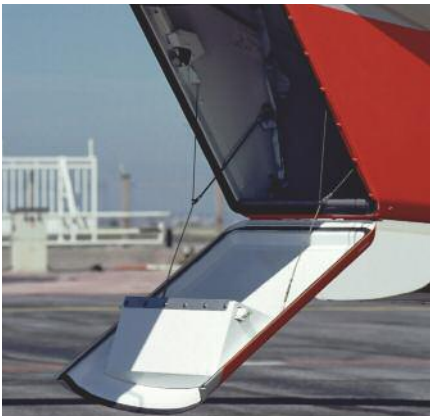
Enlarged aft fuselage compartment &amp; special one-step door
