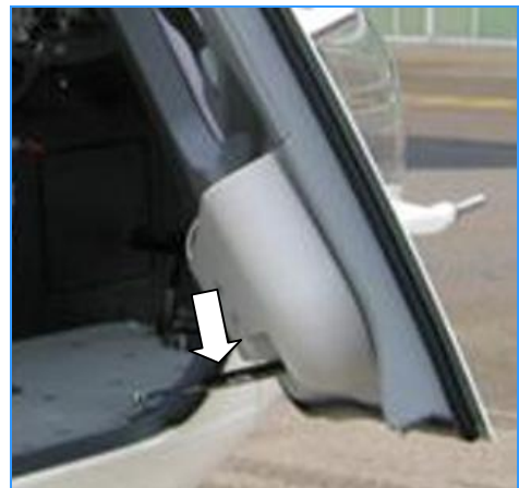
To enlarge the door opening, unhook the gas pressure spring.
