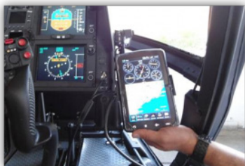
H155 panel equipped with Power outlet 28VDC
